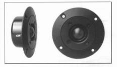
The carefully designed "catenary" profile of this critically damped, soft textile dome allows clarity of sound reproduction, together with high efficiency from 4 kHz to 20 kHz ± 2 dB, high power handling capacity of 70 Wms. Easily coupled with 2nd order crossover as shown Fig. 1. Nov crossover points are suggested for adequate power handling.
