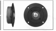
Pure Titanium is ion deposited onto an advanced soft polymer 1<sup>st</sup> diaphragm. The composite created offers increased stiffness with high internal damping, combining advantages of pure metal domes while retaining the low distortion of soft domes. The result is a detailed and musical sound reproduction Easily coupled with 2nd order crossover as shown Fig 1. Two crossover points are suggested for adequate power handling.
