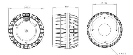
• Time coherent coaxial ring radiator design
