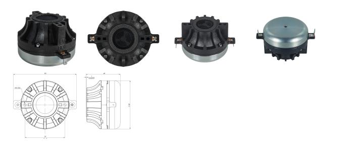
Very Compact 69 mm diameter 80 W\* continuous program power capacity 1" horn throat diameter 44 mm (1.7 in) aluminium voice coil HT Polymer diaphragm 1000 - 18000 Hz response 110 dB sensitivity Small heat sink required for full power application
