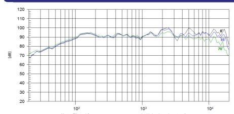
**Note:** Filtered frequency response measured with loudspeaker standing on infinite baffle in anechoic chamber, 1W @ 1m with FD-2CX
