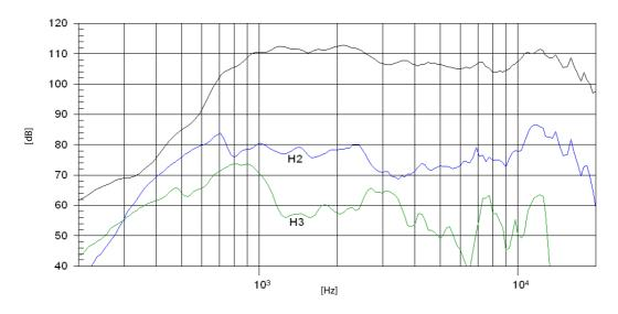
Note: On axis frequency response measured coupled to TD-385 horn in anechoic chamber, 2,83 v @ 1m  $\,$
