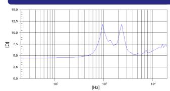
Note: Electrical impedance measured coupled to TD-385 horn
