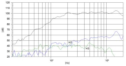
Note: On axis frequency response measured in anechoic chamber, 1W @ 1m
