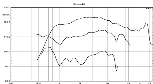
BMS 5531ND-8, 90°x75° horn, 2nd + 3rd harmonic raised 10 dB, SPL 10W / 1m
