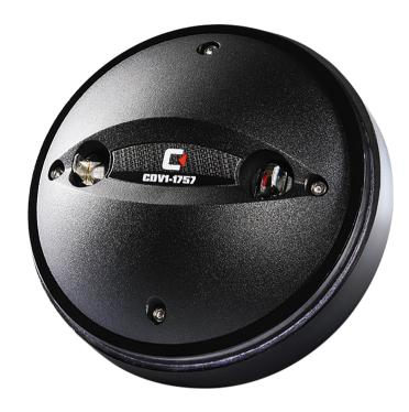
Enhanced performance in the vocal range for added clarity and intelligibility Single piece polyimide diaphragm and surround delivers low noise high output performance Proprietary Sound Castle™ diaphragm clamping system for superb reliability 800Hz recommended minimum crossover frequency (12dB/oct)
