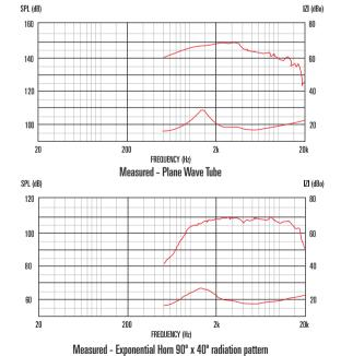
1. Tested for two hours on plane wave tube using a continuous, band-limited pink noise signal as per AES standard. Power calculated on minimum impedance. 2. Measured on axis at 1W, 1m, using typical hom, in  $2\pi$  anechoic environment.
