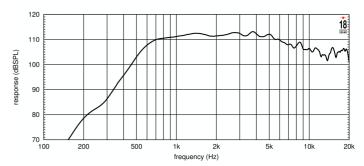
FREQUENCY RESPONSE MEASURED WITH 2,83 V INPUT ON AXIS AT 1 METER DISTANCE FROM THROAT OF XR1464 HORN.
