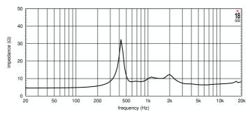
IMPEDANCE CURVE MEASURED WITH ,5 V. DRIVER MOUNTED ON XR1464 HORN.
