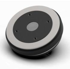
Cmp50\_vPA-S is a compression driver dedicated to high quality monitoring systems (typically high efficiency, 2 ways). The motor structure uses a 134mm diameter Ferrite magnet (grade Y40), optimized pole pieces design made of low carbon steel, and it is demodulated by Aluminum ring.
