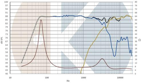
On IEC baffle / Distance: 1m / Signal input: 2,83V / At 10° Impedance measured in free air / Smoothing: 1/6 Octave Curve below 180Hz is simulated in 4.5L vented enclosure, Fc = 60Hz **NOTE:** These measurements are proceeded on IEC baffle. Some deviation could be noticed with
