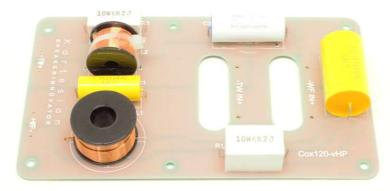
This crossover has been designed to preserve the impulse response. The filter on the woofer works as a cut-band to preserve the phase. The high-pass filter is a 2nd order, and it is built with high quality silver capacitor. The PCB size and screw holes are suitable for Kartesian terminal (separately sold). Woofer and Tweeter inputs must be connected in parallel for single wiring is used.
