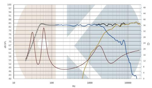
Kourtisane 4.2 / Distance: 1m / Signal input: 2,83V / On axe Impedance measured in Kourtisane 4.2 / Smoothing: 1/6 Octave Curve below 150Hz is simulated in 5.5L vented enclosure, Fc = 48Hz (Kourtisane 4.2)
