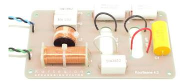
This crossover is dedicated to Kourtisane 4.2 loudspeakers kit. It works with Sub120\_vHP (or Sub120\_vHP-F) and Twt28\_vHP. Low-pass filter is 1<sup>st</sup> order with impedance correction. High-pass filter is a 3<sup>rd</sup> order with L-Pad attenuation. High quality capacitors are used for the high-pass filter.
