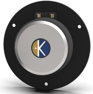
28mm soft dome designed to provide the best performances in its price range. Thanks to the technical innovation, it challenges many more expensive competitors. Very clear and detailed sounding. We recommend to use this tweeter from 2500 with 12dB/Oct. high-pass filter.
