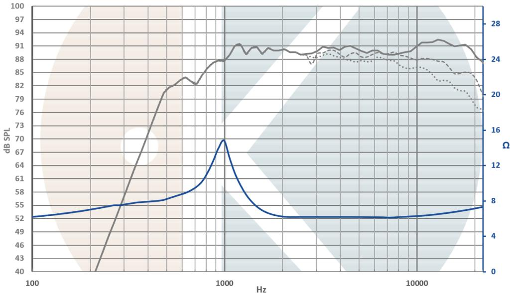
On IEC baffle / Distance: 1m / Signal input: 2,83V / High pass filter at 500Hz (48dB/Oct)
