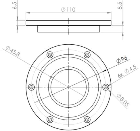
This horn provides higher sensitivity to the Twt30\_vMS in the mid-band.
