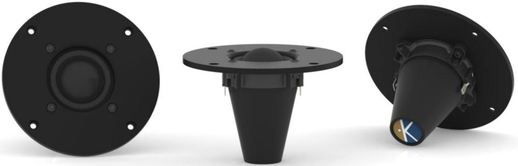
Twt30\_vMS is a sublime 30mm soft dome with large surround, dedicated to uncompromising 2 ways systems. It covers the frequency range from 1,2kHz to 22kHz (+/-2dB) with an impressively flat frequency response, and very low THD rate.
