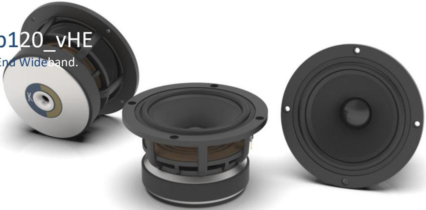
Wib120\_vHE is a modern wide band, allying low frequency extension and linear frequency response up to 22kHz. The cone (exponential profile) is made of mixed cellulose and glass fiber, with specific damping applied on the back of the membrane to minimize sound coloration.
