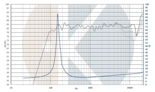
On IEC baffle / Distance: 1m / Signal input: 2,83V / High pass filter at 90Hz (48dB/Oct)
