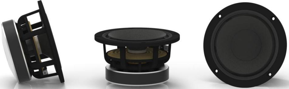
Wom120\_vMS is a very high quality mid-woofer, with extreme linearity and low distortion from 60Hz to 4000Hz. It uses the advanced hexaKone, made of treated paper with embossed honeycomb structure. The suspension is assembled on the back of the cone to avoid any diffraction out of axe. The magnetic system has been engineered with FEA and it uses a long cooper ring to minimize inductance effects.
