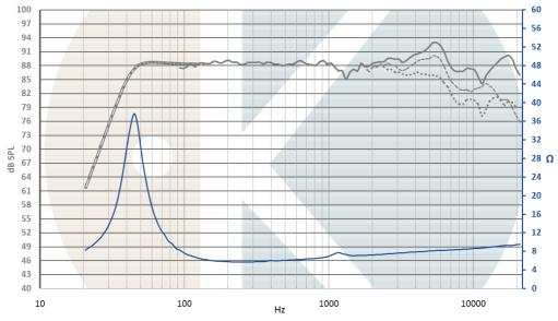
On IEC baffle / Distance: 1m / Signal input: 2,83V / Dash curves: 30° & 60° Impedance measured in free air / Smoothing: 1/12 Octave Curve below 130Hz is simulated in 16L vented enclosure, Fc = 43Hz
