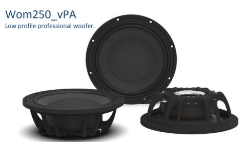
Wom250\_vPA is engineered to cover 50 - 850Hz (-3dB) in a very compact enclosure (sealed or vented). The advanced motor structure is built with Ø116mm voice coil, high grade ferrite magnet and it is demodulated by 2 Aluminum rings.
