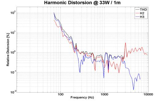
Non linear curves measured thanks to Klippel software and hardware, in free air
