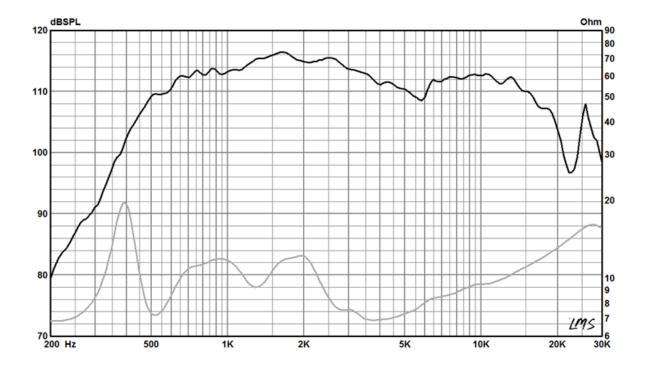
Frequency response and impedance of 950NeoBePB-16 on specified horn, free field <sup>3</sup>.
