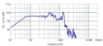
Frequency response curve of the loudspeaker make in a hemispherical, free field applying a sinusoidal signal of 2.83 V @8 at 1m.
