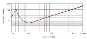
Impedence magnitude curve measured in free air
