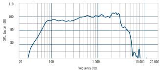
Frequency response curve of the loudspeaker made in a hemispherical, free field and mounted in a reflex box with an internal volume of 50 litres and tuned at 60Hz, applying a sinusoidal signal of  $2.83\,\text{V}\otimes8$  at  $1\,\text{m}$ .
