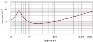
Impedance magnitude curve measured in free air.
