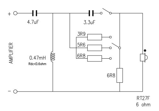
All resistors must be minimum 4Watt Metal Oxide type. All capacitors must be Polypropylene foil type, 160V rating.
