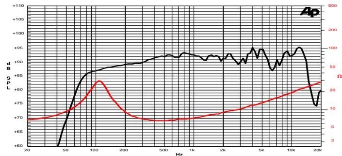
Frequency Response on 10 Lt @ 75 Hz Vented Box @ 1W, 1m
